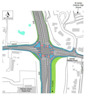
The A34 has a four-arm junction with Stanley Road, controlled by traffic lights. Pedestrians and cyclists would be able to cross the A34 in stages using controlled crossings. This option has more crossing stages for pedestrian and cyclists, making it more complex to cross.
